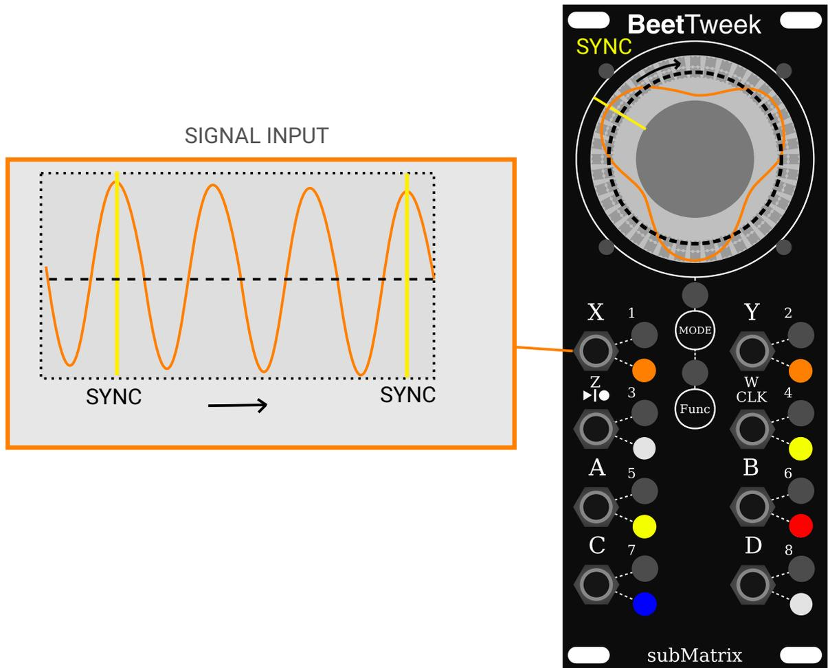
Regions where the SIGNAL INPUT is further away from the HAPTIC KNOB are regions where the TORQUE applied to the knob will be POSITIVE. Regions where the SIGNAL INPUT is closer to the HAPTIC KNOB are regions where the TORQUE applied is NEGATIVE. Regions where the SIGNAL is near the dotted line are regions where ZERO TORQUE will be applied.
