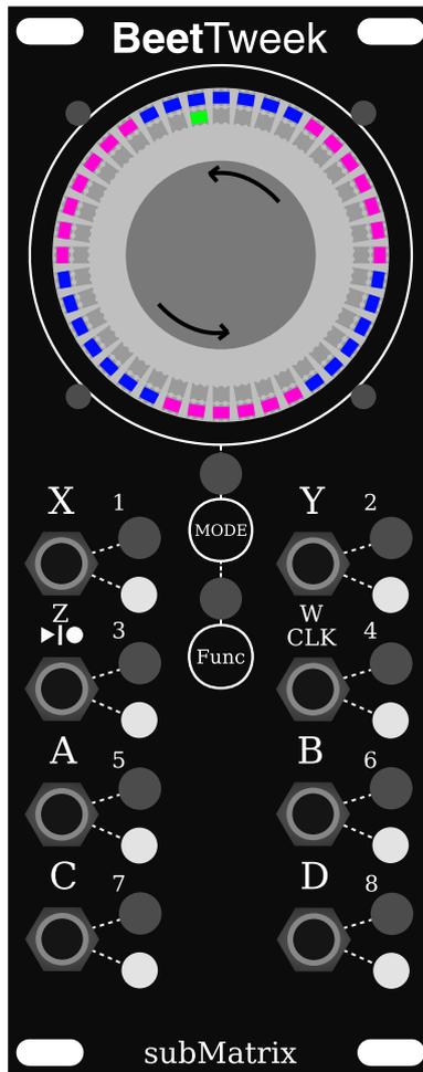
The current TORQUE is available on output **A**, while the current ANGLE is available on OUTPUTS (**B** and **C**). The SIGNAL INPUT is a summation of inputs (**X** and **Y**). The SUM is passed through an internal HIGH-PASS filter to remove DC bias, the AMPLITUDE of the signal is tracked continuously and then scaled to compensate internally.
