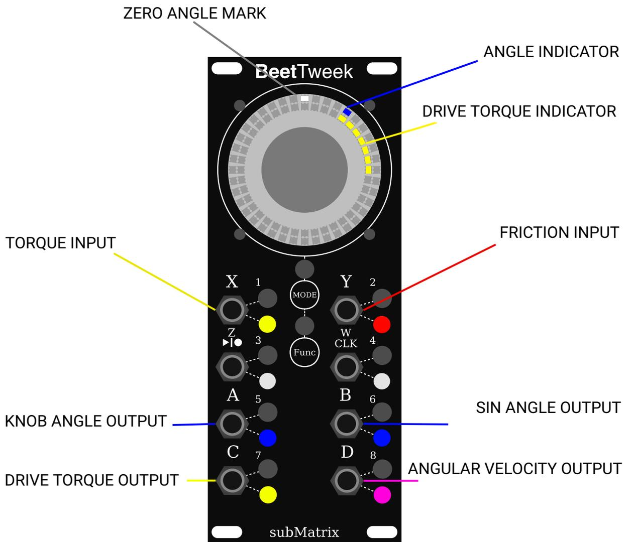
The TORQUE INPUT (X) drives the HAPTIC KNOB CLOCKWISE and COUNTER-CLOCKWISE with torque proportional to the input voltage. The DRIVE TORQUE INDICATOR indicates the direction of this torque around the knob as well as
