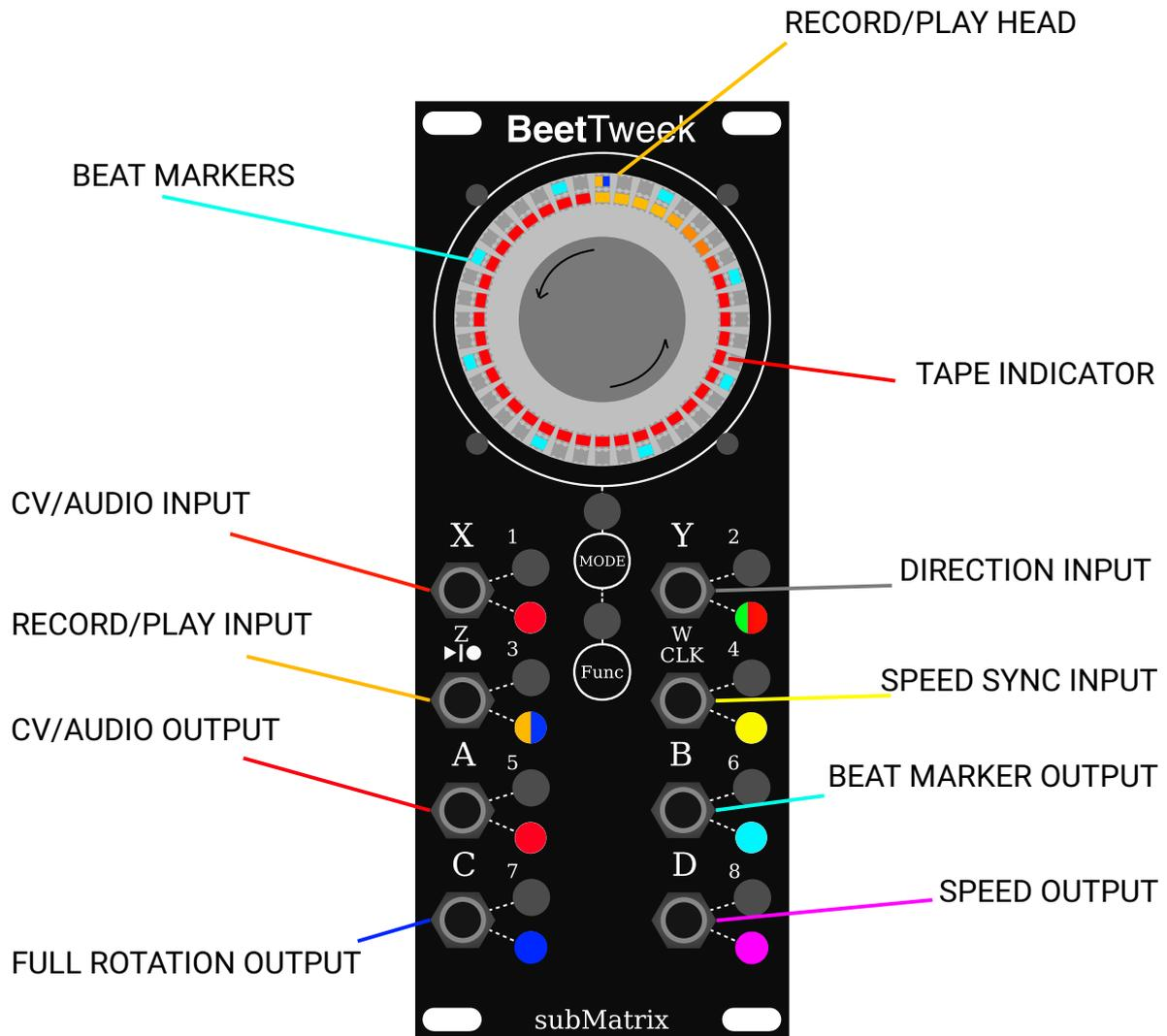
The RECORD/PLAY INPUT ( $\frac{Z}{\blacktriangleleft \bullet}$ ) is used to RECORD or PLAYBACK signals from the CV/AUDIO INPUT (X). The RECORD/PLAY INPUT is a GATE signal that is in RECORD Mode when the SIGNAL is Less than 2.5V and PLAY mode when the signal is greater than 2.5V.
