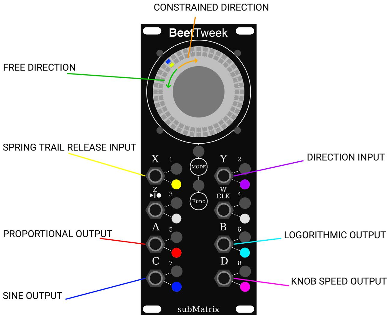
When the HAPTIC KNOB is rotated in the CONSTRAINED DIRECTION. A SPRING TRAIL begins to form on the inner LED RING indicator. A COUNTER-TORQUE is applied to the HAPTIC KNOB as the SPRING TRAIL extends in length. The Length of this trail (Donated  $D$ ) controls the OUTPUTS (A,B and C).
