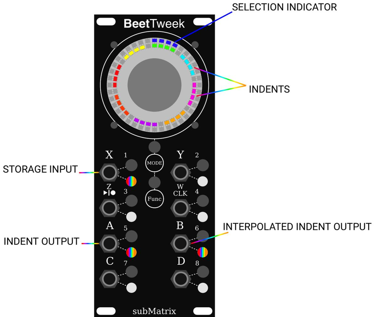
The SELECTION INDICATOR indicates which INDENT the HAPTIC KNOB is Currently Snapped To. Turning the knob will rotate the SELECTION INDICATOR around the circle. As the knob rotation from INDENT to indent, HAPTIC Forces will snap the knob to the INDENT angle locations.
