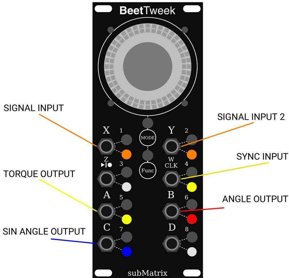
In this mode, a waveform from another module is fed into the SIGNAL INPUT (X+ Y). The wave form is then captured in a manner similar to an oscilloscope, where the SYNC INPUT ( $\frac{W}{CLK}$ ) is used to capture a synchronized window of time from the SIGNAL INPUT. The SYNC INPUT is a GATE signal that starts capturing the SIGNAL when the voltage goes from 0v to 5v. For repeating wave-forms, the SYNC INPUT should be in sync (within some multiple) of the SIGNAL INPUT.
