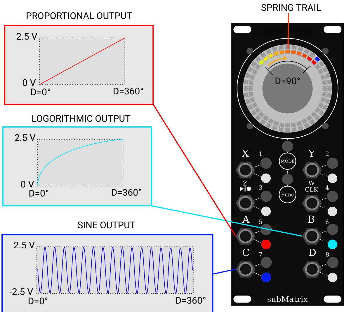
The SPRING TRAIL can be dynamically shortened in length by using the **X** INPUT. The Higher the Voltage value the faster the SPRING TRAIL will retract back to length 0.
