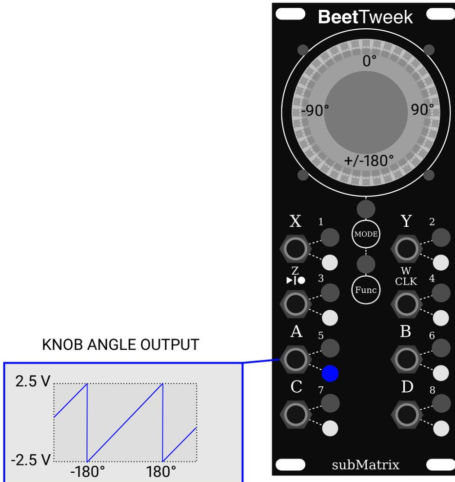
The SIN ANGLE OUTPUT (**B**) Outputs a voltage proportional to the sin of the current angle of the HAPTIC KNOB, and will cycle every 360 degrees:
